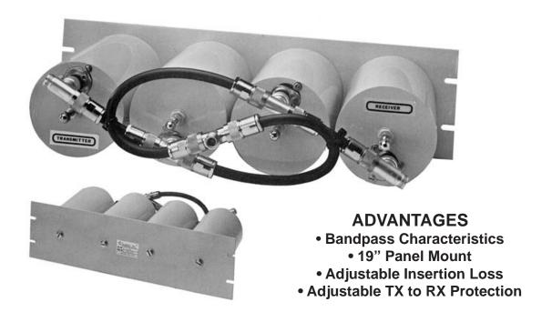
The TELEWAVE TPRD-4544/4744 Base Station Duplexers set an all-time standard for the LMR industry. By using two TPRC-4504 or 4704 Bandpass/Band-Reject cavities in each transmitter and receiver path, these duplexers provide maximum TX to RX protection in the most severe RF environments.
